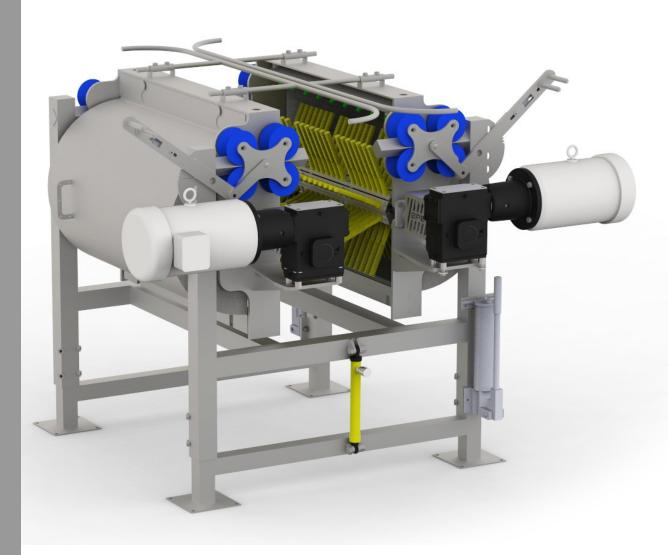
The Berry Wing Picker B-WP-4-48 is designed to clean the wings by the rotating rubber fingers which are placed to gently brush away cuticle matter, then rinse the matter away with use of the water spray nozzles. The model B-WP-4-48 is constructed of stainless steel, Teflon, and aluminum for durability and easy clean up and has the capacity to process up to 300 birds per minute. The model B-WP-4-48 should be positioned after the last bird picker on the picking line.
