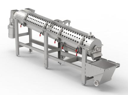
The Berry Plumbing & Equipment Foot Picker is constructed entirely of stainless steel, aluminum, and rubber for durability and easy cleanup. Paws from your Berry Paw Harvester are transported to the Berry Foot Picker where they are fed into the infeed chute. The paws fall into a picking chamber where a rotating system of fingers gently push them against a bank of fixed fingers above while moving them steadily downward to the discharge chute where they emerge clean and cuticle free.
