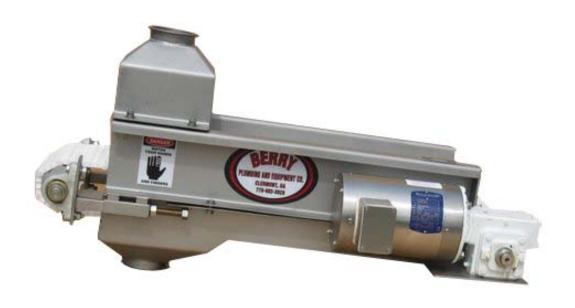
The Berry Plumbing & Equipment Dewatering Conveyor 2 is constructed entirely of stainless steel and UHMW aluminum for durability and easy cleanup. Pump fed and electrically powered, installed after the foot picker but before the final inspection table, the Dewatering Conveyor 2 features a moving belt that allows water to drain off the paws before the product reaches the inspection table.
