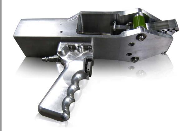
Berry's **Finger Master 5000, Model B-FM-5000** is an innovative pneumatic tool used to pull picking fingers in to the finger bank. The time savings are phenomenal, a job that would normally take three hours will now only take forty-five minutes. Every piece of the Finger Master is precision made out of the highest grade of non-corrosive material that gives you longevity and quality that can expect with the Berry name.
