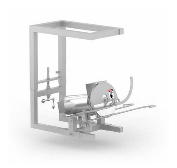
Model **B-HS-1 Halving Saw** from Berry Plumbing & Equipment Company, allows vertical, horizontal and tilt adjustment of the blade for precise cutting, while the unique guide bar configuration directs the wings away from the blade, increasing 'A Grade' wing yield.
