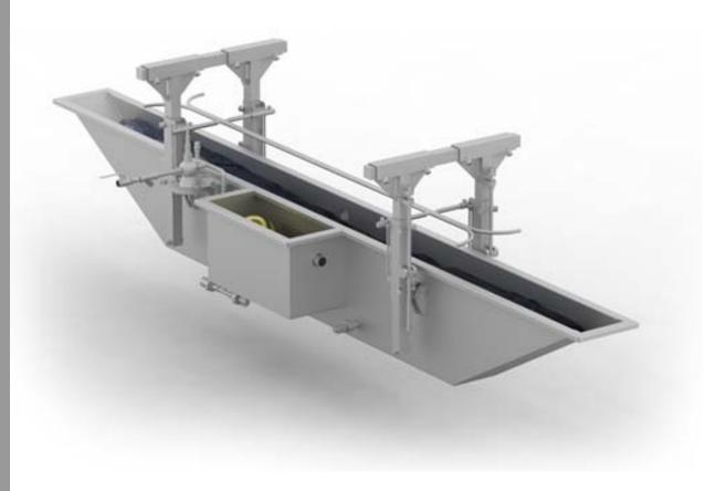
The Model **B-DTS-9 Berry Dip Tank Scalder** is being used in Paw Harvesting operations on the return line. While remaining on the shackles, the paws are immersed into the tank as the steam injected hot water softens the paws which aids in the removal of cuticle and ammonia burns.
