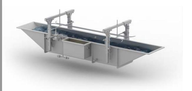
The Model **B-DTS-DL-9 Berry Dip Tank Scalder with Dual Lane capacity** is being used in Paw Harvesting operations on the return line. While remaining on the shackles, the paws are immersed into the tank as the steam injected hot water softens the paws which aids in the removal of cuticle and ammonia burns. This pre-heating method may also be used on Wings to soften cuticle and feathers for easier removal.
