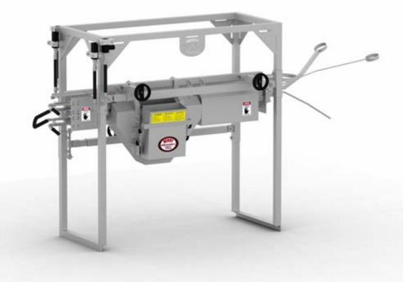
Automatically fed, hydraulically powered and designed to remove the paws of all size birds lots, **Model B-PH-EXT-48-LH/RH Paw Harvester** from Berry Plumbing & Equipment will handle any line speed and provide a significant increase in yield.
