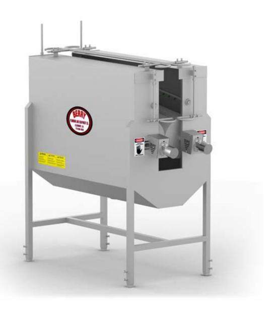
Berry's Bird / Wing Scrubber, Model B-BS-1 provides an efficient process to remove fecal matter from defeathered birds. Hydraulic motors rotate the nylon brushes in a downward motion, gently scrubbing and removing fecal matter, as the bird travels through the Bird Scrubber Model B-BS-1. In both sides of the Scubber, a water rail with spray jets rinses away fecal matter and debris while continuously rinsing the brushes.
