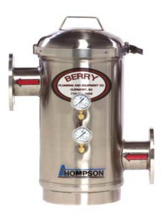
The **Berry/Thompson Water Strainer** is designed to remove most remaining particles that are left in the water after filtering through the water screen. Particles are then automatically flushed out to drainage, and the re-usable water is pumped back in to the plant. This process prevents any nozzle stop-up from occurring.
