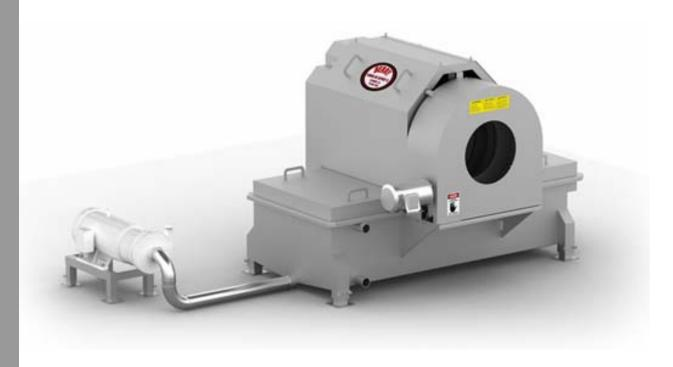
The Berry Water Re-Use Screen is designed to filter out all heavy solids, separating them from the water coming from the final bird washers and reusing that water in various areas throughout the plant. The screen is made up of stainless steel construction and is gear to gear driven. Capable of recycling up to 200 gallons of water per minute, the Water Re-Use Screen set up has a tank with a fresh water make-up float valve and is connected to a pump also rated at 200 GPM.
