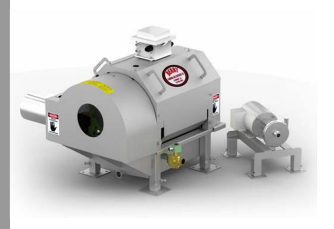
The Berry Water Re-Use Screen is designed to filter out all heavy solids, separating them from the water coming from the final bird washers and reusing that water in various areas throughout the plant. The screen is made up of stainless steel construction and is gear to gear driven. Capable of recycling up to 60 gallons of water per minute.
