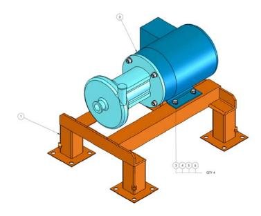
Pump and Motor assembly for pumping recycled water from Berry Water Reuse Screen BWS6-60 to desired reuse area in plant.
