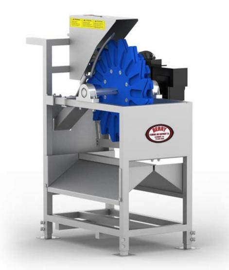
Model **B-WM-1** is designed to give you quality cuts on the three sections of the wing leaving you with top grade maximum yield on the drumettes, flats (2nd portion), and tips. The unique 3 piece wing wheel allows customers to purchase only the worn out section of the wheel, rather than purchasing and replacing an entire wheel.
