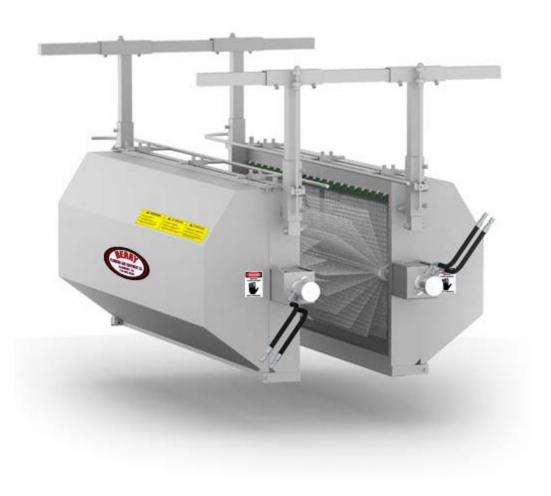
Hydraulic or electric motors rotate the nylon brushes in a downward motion, gently scrubbing and removing fecal matter and cuticle as the overhead conveyor carries the bird through the **Bird/Wing Scrubber B-BS-2-96**. In both sides of the scrubber, a water rail with spray jets rinses away fecal matter and debris while keeping the brushes clean. Two sets of horizontally and vertically adjustable guide bars keep any size bird stable as it is cleaned.
