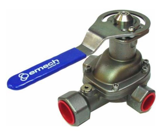
The shear action disc design provides precise control mixing of steam and water. Fitted with an electronic actuator, and integrated temperature sensor results in fast, accurate and stable temperature control. As a single compact assembly, installation is simplified. The independence of this stand alone unit provides a reliable solution of hot water supply.
